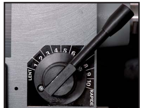
10 Vitesses variables de 500 à 2000 tr/min 10 speeds ranging between 500 to 2000 tr/min
